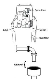
**Outlet:** This is the softened water leaving the softener to supply the rest of the house.
