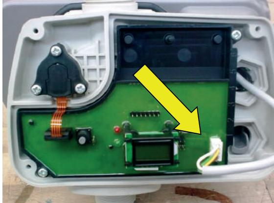
*Disconnect the wire communication with the power board*
