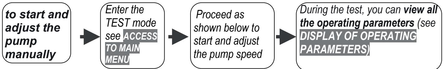
**CAUTION: TEST mode is not active on the SLAVE unit; to make a TEST on the SLAVE unit, switch off temporarily the MASTER unit, so that the SLAVE unit becomes independent and is able to perform the TEST normally**
