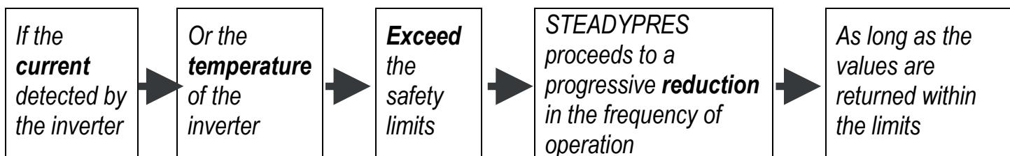
While operating in self-limitation, DISPLAY and LED flash to indicate the fault status
